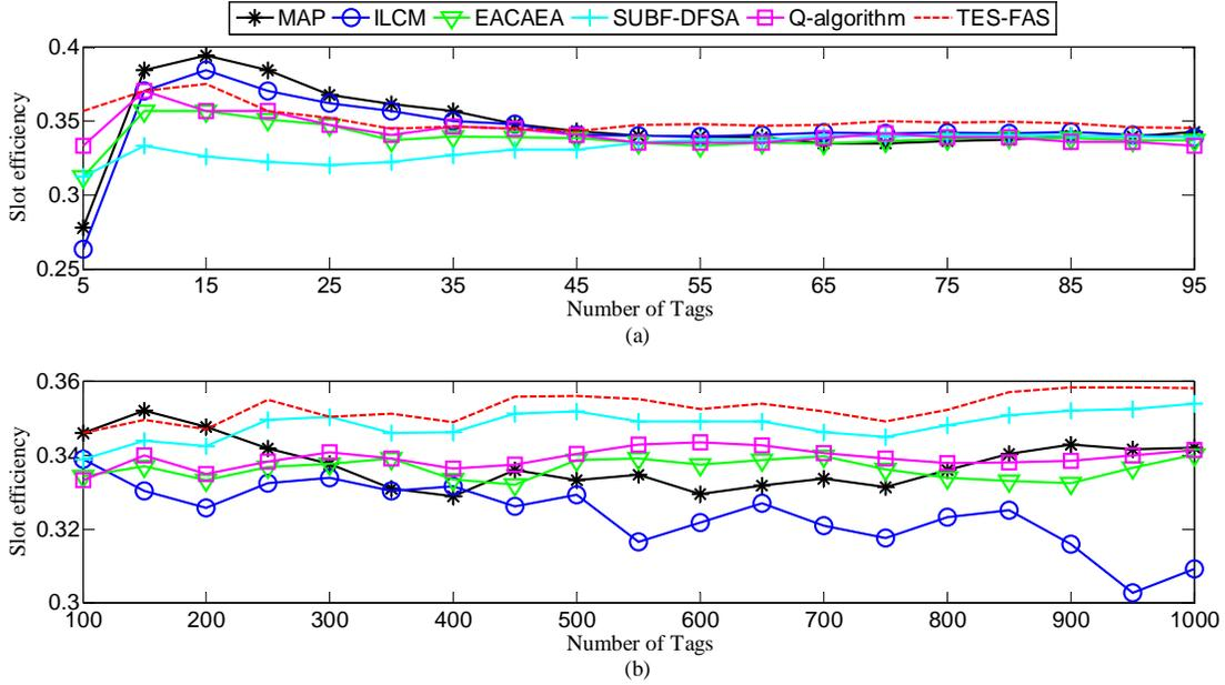
Fig. 2. The comparison of slot efficiency: (a) for  $5 \leq n \leq 95$  (b) for  $100 \leq n \leq 1000$
