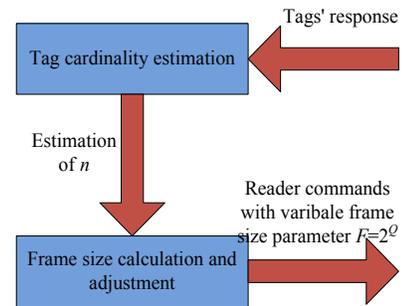
Fig. 1. The DFSA protocol for reader operation
