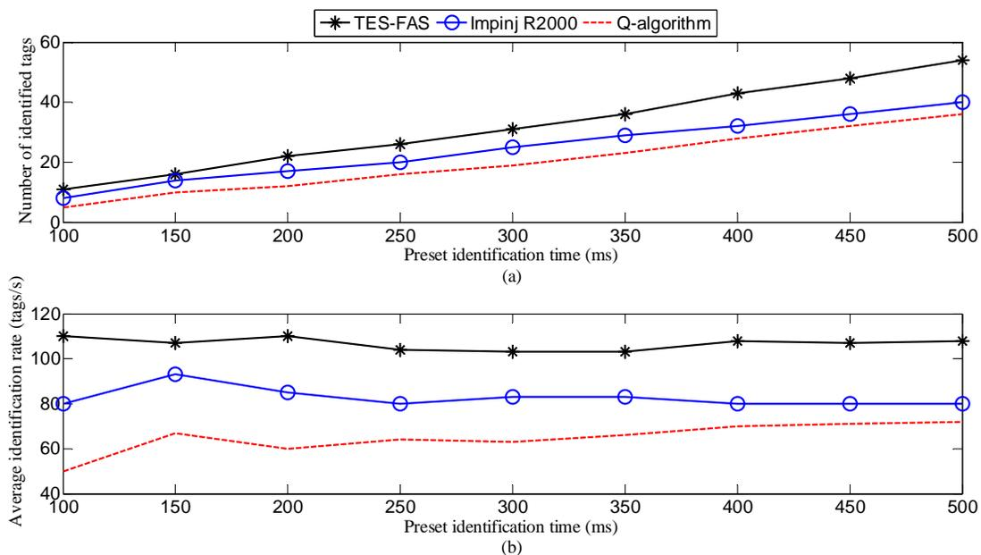
Fig. 8. Comparison of the experimental results under scenario 2: (a) number of identified tags (b) average identification rate
