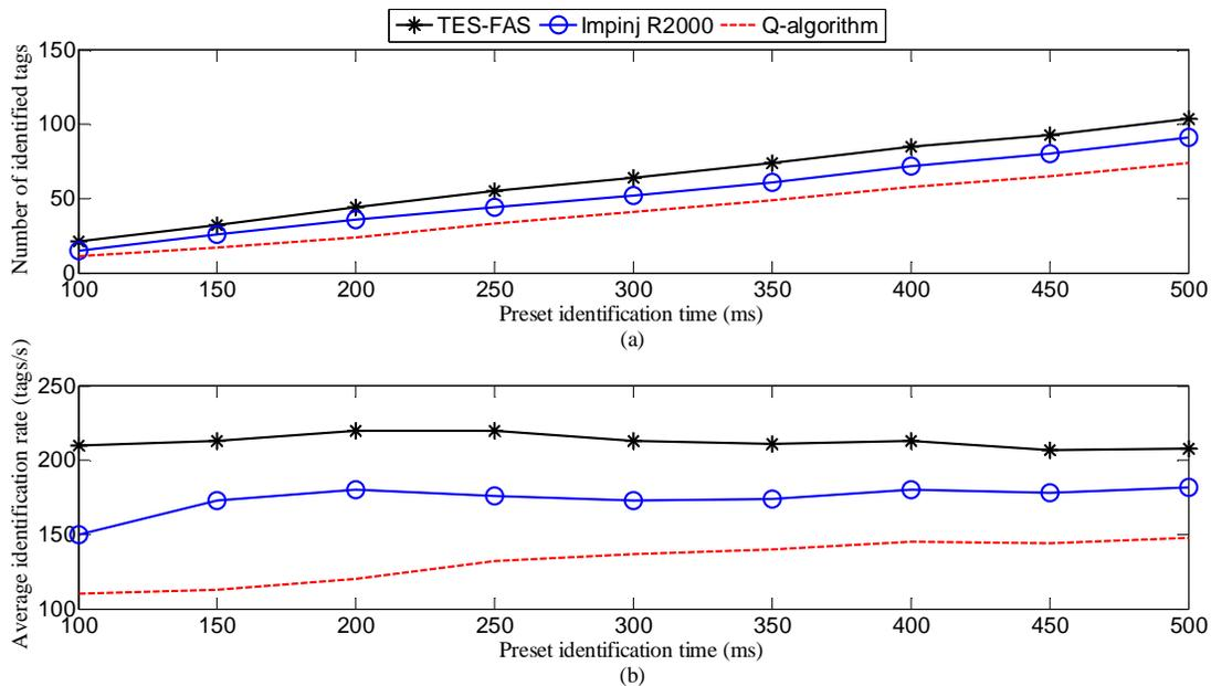
Fig. 7. Comparison of the experimental results under scenario 1: (a) number of identified tags (b) average identification rate
