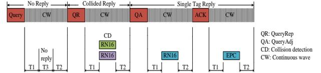
Fig. 1. Link timing between a reader and tags
