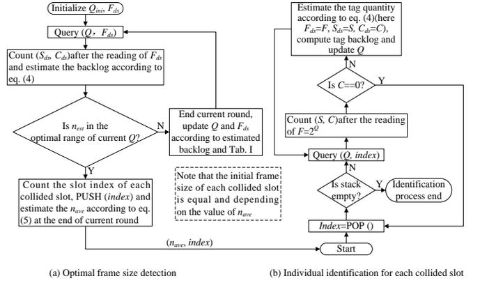
Fig. 2. The flowchart of the proposed ds-DFSA
